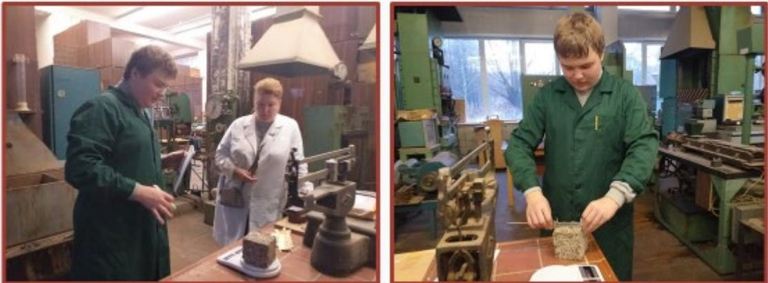
The image contains two photographs. The left photograph shows a young man in a green lab coat measuring the dimensions of a rectangular arbolite sample on a workbench. A woman in a white lab coat is standing nearby. The right photograph shows the same young man weighing the arbolite sample on a scale.
