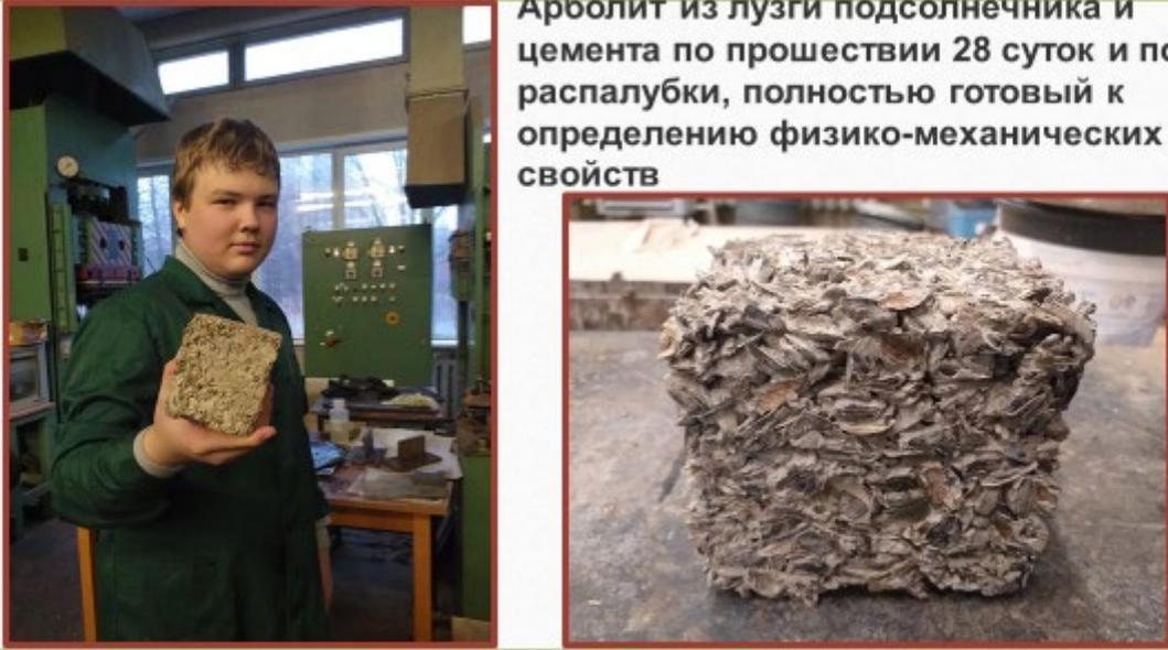
The image shows a young man in a green lab coat holding a rectangular sample of arbolite. To his right is a close-up photograph of a large, textured, cylindrical block of arbolite, which is a composite material made of sunflower husks and cement.
